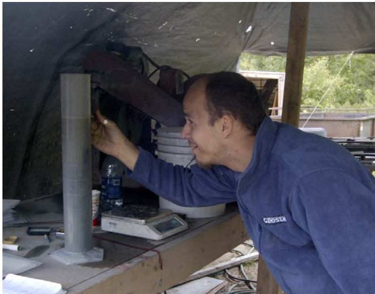
Figure 46: Measure of the volume of the rock samples for determination of the density
