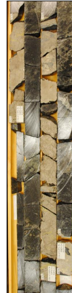
Diamond drill core from DDH97-067 with 1.97% Ni, 1.03% Cu, and 0.26% Co over 60 cm.
