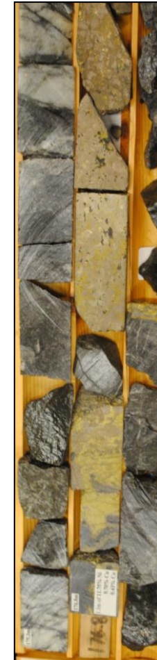
Diamond drill core from DDH97-075 with 11.6% Ni, 10.2% Cu, and 0.41% Co over 1.1 m.
