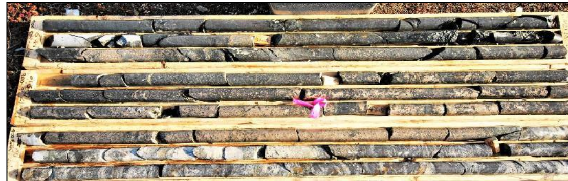
DDH 17-6 45.3m to 49.2m: 3.9m @ 0.37% Ni, 0.10 % Co, 0.27% Cu
