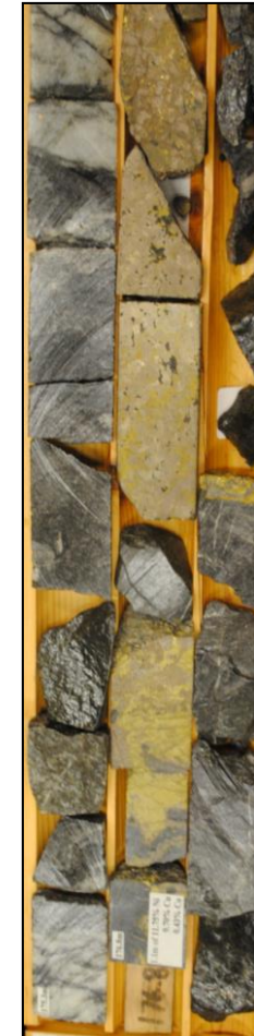
Diamond drill core from DDH97-075 with 11.6% Ni, 10.2% Cu, and 0.41% Co over 1.1 m.
