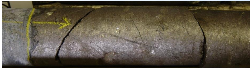
SVB-02-138, 297.74-298.51 m: Massive sulphide vein in footwall 0.77 m @ 1.37% Ni, 0.64% Cu SOUTH GABBRO
