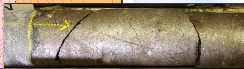
SVB-02-138, 297.74-298.51 m: Massive sulphide vein in footwall 0.77 m @ 1.37% Ni, 0.64% Cu SOUTH GABBRO
